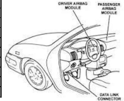
As American Honda Motor Company, Inc. and NHTSA have publicly advised, in certain vehicles, the passenger and/or driver frontal airbag inflator could produce excessive internal pressure. If an affected airbag deploys, the increased internal pressure may cause the inflator to rupture. In the event of an inflator rupture, metal fragments could be propelled upward toward the windshield, or downward toward the front foot well, potentially causing injury or fatality to vehicle occupants.
